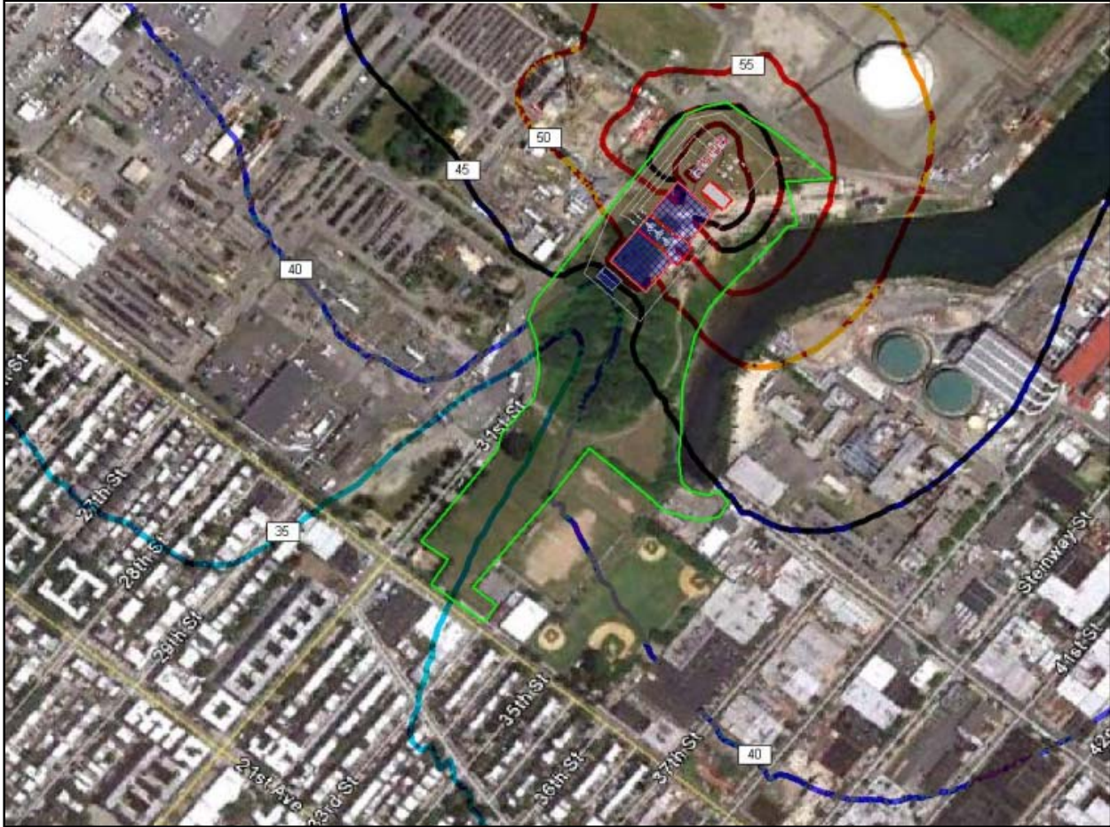
Figure 5.4.17-1. Noise Contour Map of Predicted Noise Associated with Operations of the Luyster Creek Converter Station
